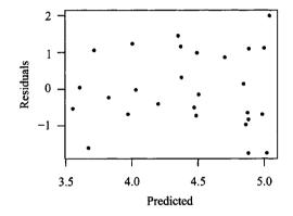
**Figure 6.18** Plot of standardized residuals against the fitted values when  $\ln Y$  is regressed on X and  $X^2$ .
