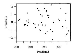
Figure 7.10 Standardized residuals versus fitted values for WLS solution.
