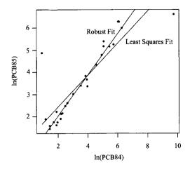
**Figure 13.3** Least squares and robust fits superposed on scatter plot of  $\ln(PCB85)$  versus  $\ln(PCB84)$  for the data set in Table 13.7.
