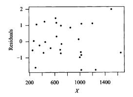
**Figure 6.19** Plot of standardized residuals against X when  $\ln Y$  is regressed on X and  $X^2$ .
