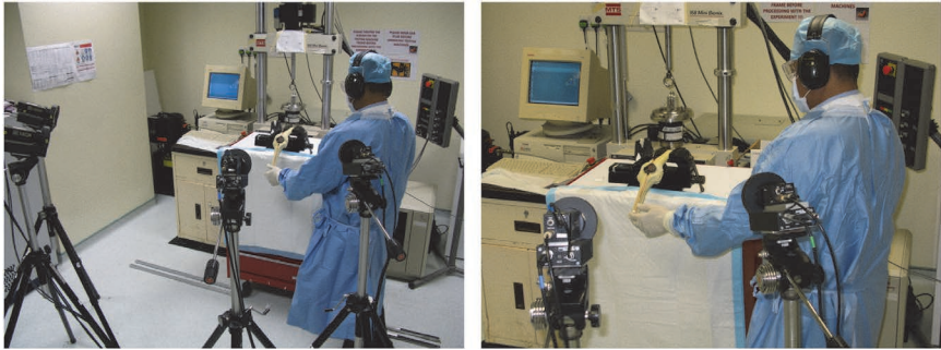
Fig. 6.22: Stimulating knee model range of motion with Vicon motion capture cameras used to track 3D motion.
