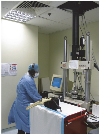
Fig. 6.23a: Operating the MTS 858 Mini Bionix testing machines with compressive, tensile and torsional testing functionalities.
